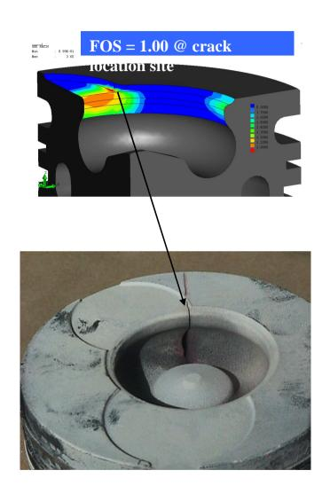
Piston is essentially trying to bend around the steel pin High mechanical stresses on bowl and pin hole
