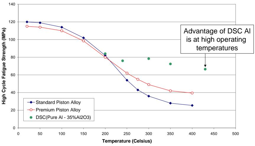
A huge improvement over current premium piston alloys at elevated temperatures. Increases in low temperature fatigue strength will be obtained with an alloyed matrix rather than pure Al
