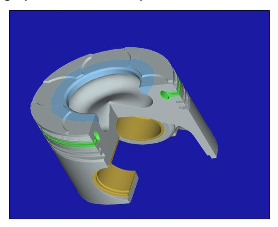
Bowl edge insert using DSC Aluminium is the logical way forward Only use it where it is needed to keep costs down!
