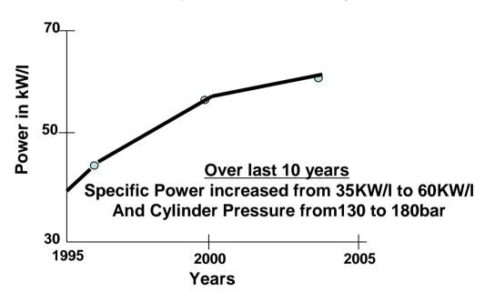
**Engine downsizing is continuing! Further reduction of oil consumption** Particulate filters Multi point injection
