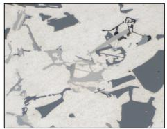
Very much finer microstructure in DSC AI than in standard cast piston alloy
