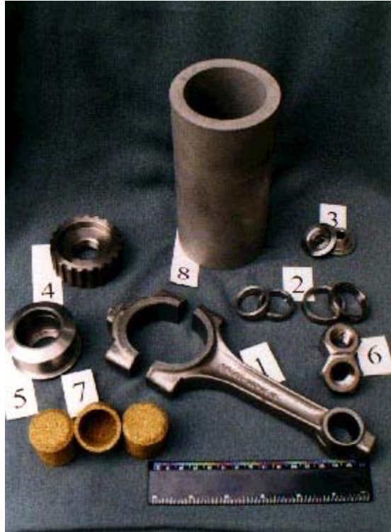
Figure 13. Ti-6Al-4V parts produced using a press-and-sinter approach and titanium hydride. 1) Connecting rod with big end cap; 2) Saddles of inlet and exhaust valves; 3) Valve spring plate; 4) Distribution shaft driving pulley; 5) Strap tension gear roller; 6) Screw nut; 7) Fuel pump filter; and 8) Embedding filter.
