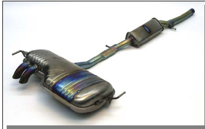
Figure 9. Exhaust system for the Golf 4motion, CP titanium, approximately 50% weight reduction compared to a steel component.
