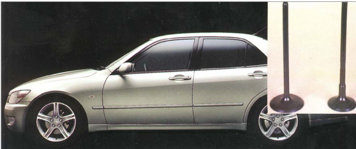
Figure 7. The Toyota Altezza, 1998 Japanese Car of the Year, the first family automobile in the world to feature titanium valves. Ti-6Al-4V intake valve (left) and TiB/Ti-Al-Zr-Sn-Nb-Mo-Si exhaust valve (right). (Courtesy Toyota Central R & D Labs, Inc.).
